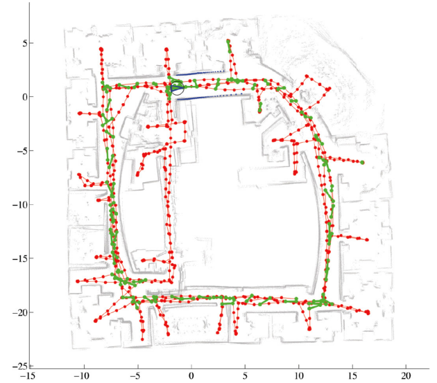
Fig. 14. Filtered trajectory using encoder odometry and laser scans of the Intel dataset. Blue arrow indicates the final pose of the robot and the black ellipse the associated covariance at a 95% confidence level.
