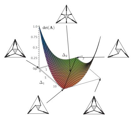
**Figure 8**. By properly choosing the offsets  $\Delta_1 = \delta_1 = \delta_3 = \delta_5$  and  $\Delta_2 = \delta_2 = \delta_4 = \delta_6$  in Fig 7, it is possible to reach architecturally singular platforms including the obvious situations in which couples of legs coincide and the architecturally singular Griffis-Duffy platform.
