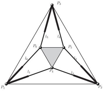
Figure 4. Octahedral manipulator and associated notation.
