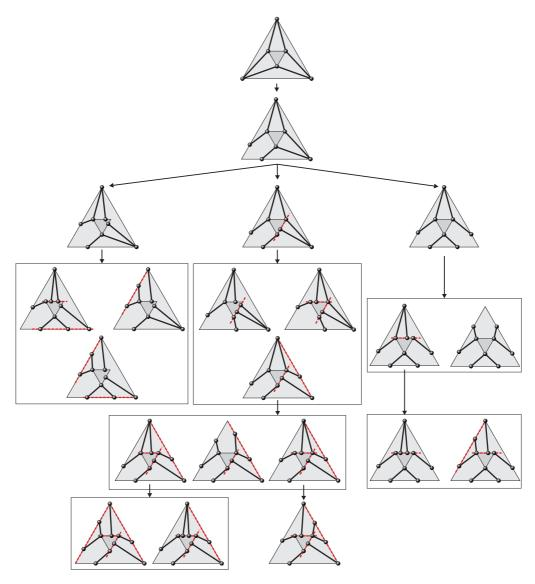
**Figure 6.** Family of manipulators kinematically equivalent to the octahedral manipulator obtained by sequentially applying the geometric transformation in Fig. 5. Dotted red lines indicate required alignments.
