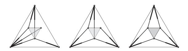
**Figure 1**. The three possible topologies for a 3-3 Stewart-Gough platform. The rightmost one corresponds to the octahedral manipulator.
