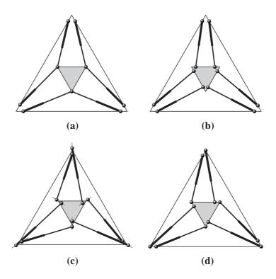
**Figure 2**. The triple arm mechanism (**a**), the standard approximation to the octahedral manipulator that avoids all double-ball-joints (**b**), the Stoughton-Arai approximation intended to also improve the dexterity of the manipulator (**c**), and the Griffis-Duffy modification (**d**).
