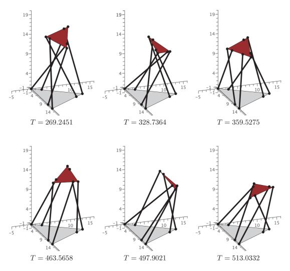
**Figure 9**. The forward kinematic solutions of the analyzed example. The mirror reflections with respect to the base plane are not included.
