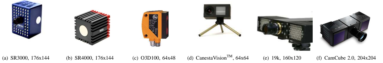
Fig. 2. Current commercial lock-in ToF cameras. (a-b) Mesa Imaging AG © [3]. (c) Ifm electronic © [4]. (d) CanestaVision TM [5]. (e-f) PMD[Vision] ® [6]. Particularities of each solution include the use by CanestaVision TM of square modulated waves [7], the use of a smart pixel - photonic mixer device (PMD) for simultaneous wave sensing and mixing by PMD[Vision] ® [8], and the addition by Mesa Imaging AG © of a coded binary sequence (CBS) modulation for multi-camera operation on SR4000 new models.
