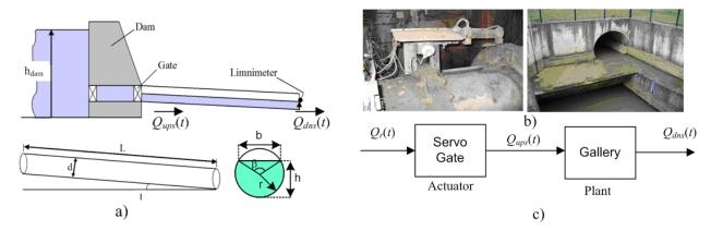
Fig. 1. Lunax gallery. a) Geometrical scheme; b) Pictures; c) Functional scheme
