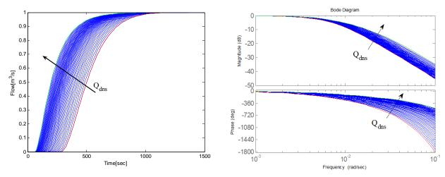
Fig. 2. (a) Step response and (b) Frequency response for different operating points
