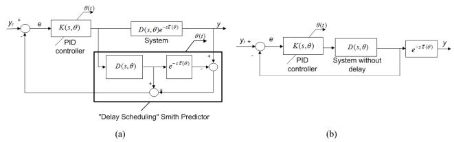
Fig. 3. (a) "Delay scheduled" Smith Predictor scheme. (b) Equivalent Smith Predictor closed-loop
