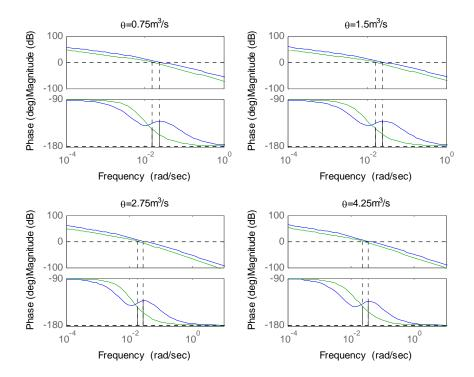
Fig. 4. Frequency response (and phase margins) of the PID (blue) and PI (green) in series with the delay-free part of the plant in the considered operating points
