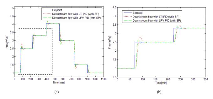
Fig. 6. (a) Closed-loop response for different operating points, using LPV and LTI control with SP. (b) Detail of the part of the closed-loop responses
