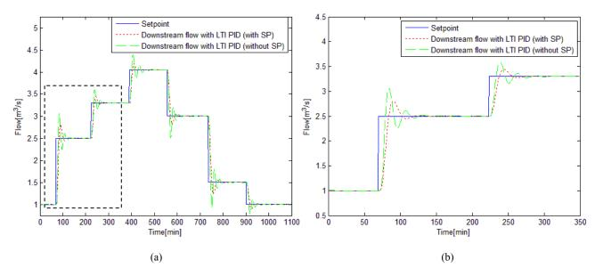
Fig. 9. (a) Closed-loop response for different operating points using LTI control with and without SP. (b) Detail of the part of the closed-loop responses.
