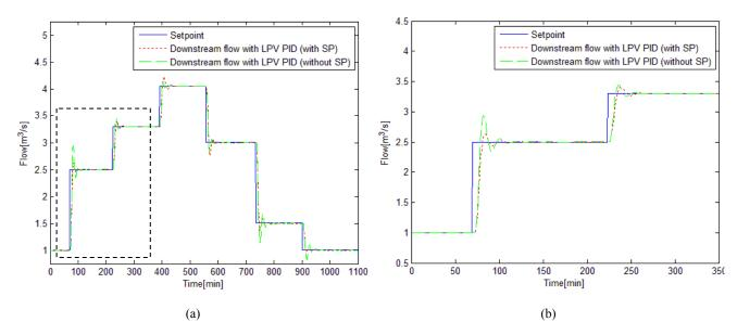
Fig. 8. (a) Closed-loop response for different operating points using LPV control with and without SP. (b) Detail of the part of the closed-loop responses.
