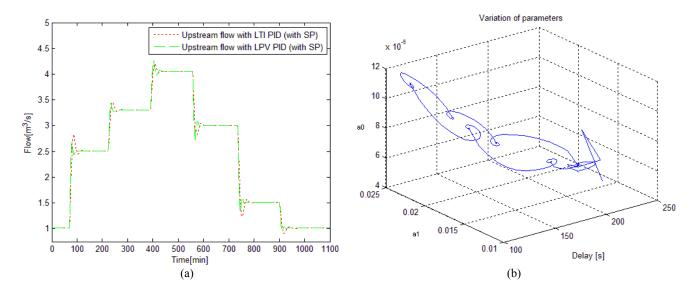
Fig. 7. (a) Control actions (released upstream flow) corresponding to the operating point changes presented in Fig.6a.
