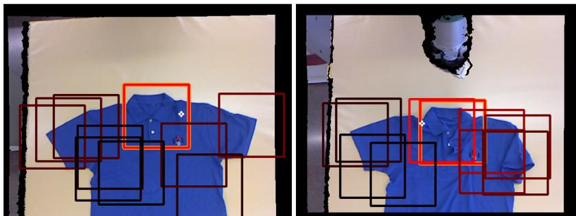
**Figure 1.** Bounding boxes and FINDDD selected grasping point. The red box contains the collar and FINDDD scores will be calculated inside it.
