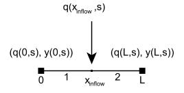
Figure 2: Water inflow flowing into a canal, leading to a simple interconnection structure.
