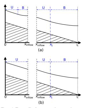
Figure 4: Flow profiles for a two-reach system when  $x_1 > x_1$  $x_{inflow}$ . (a) Independent flow profile. (b) Consistent flow profile.
