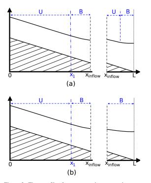
Figure 3: Flow profiles for a two-reach system when  $x_1 < x_1 < x_1 < x_2 <$  $x_{inflow}$ . (a) Independent flow profile. (b) Consistent flow profile.
