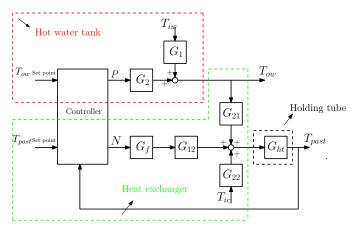
Fig. 3. Control block diagram.
