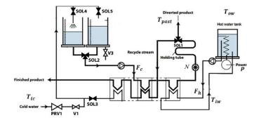
Fig. 2. Pasteurization plant scheme.
