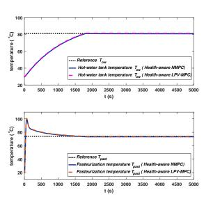
Fig. 4. Evolution of controlled temperature of health-aware NMPC strategy and the proposed algorithm.
