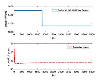
Fig. 5. Evolution of the control action of health-aware LPV-MPC.
