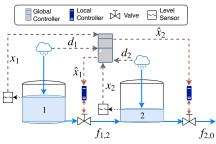
Fig. 1. Hierarchical control scheme for drainage systems adapted from [2]. A global controller retrieves information from rain and level sensors and sets the flow references for the local control level.
