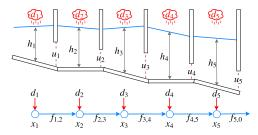
Fig. 2. Five open channels in series. The volume at each channel is controlled by using a gate. Each reservoir receives runoff water coming from the environment (red flows). The compartmental graph of the system is presented at the bottom.
