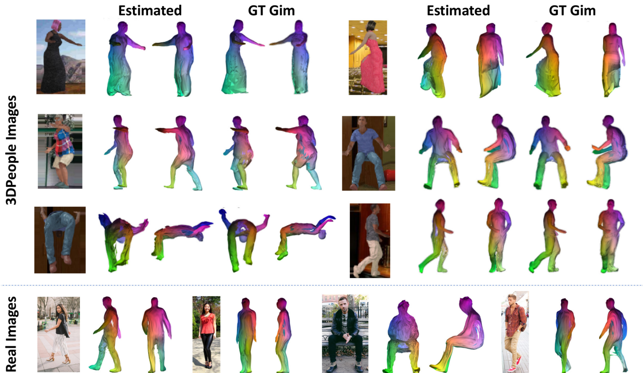
Figure 8. Qualitative results. For the synthetic images we plot our estimated results and the shape reconstructed directly from the ground truth geometry image. In all cases we show two different views. The color of the meshes encodes the xyz vertex position.
