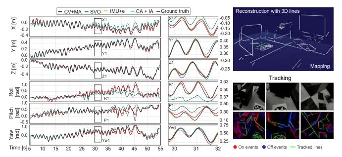
Figure 4. Trajectory and 3D reconstruction with PTAM system using CV + MA variant in *Office L shape* scenario. The tracked lines are highlighted in green in the tracking snapshots, and the line map was captured from Rviz at the end of the sequence.
