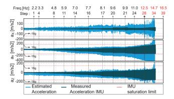
Figure 6. Linear acceleration measured and estimated during the stress experiment. Note: IMU acceleration is saturated after 750 rpm (12.5 Hz) where the camera experiences an acceleration higher than 16g
