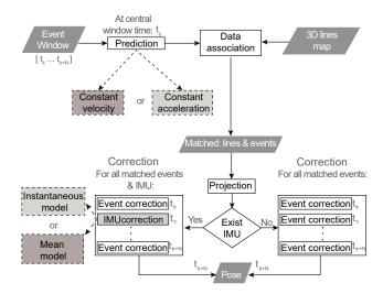
Figure 1. Strategy 1: Events and IMU in the correction stage.
