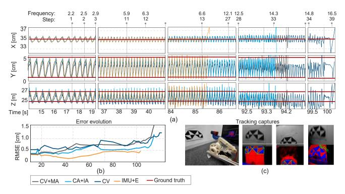
Figure 5. Position estimation in stress test from 240 rpm to 990 rpm with CV+MA, CV+IA, and IMU+e variants: (a) position estimation, (b) error evolution, (c) four-bar mechanism with tracking snapshots until the system failure.
