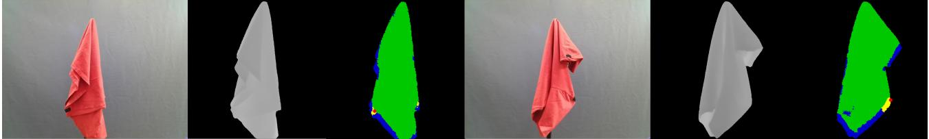
**Figure 5: Visualization of the results with a different depth camera. Background, cloth body, edges are denoted in black, green, blue respectively. Grasping points with highest confidence are highlighted by dots in red.**
