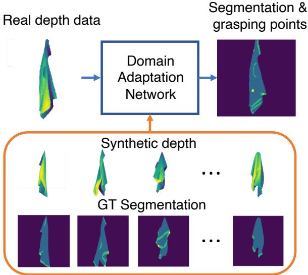
**Figure 1: Overview of our approach.** We introduce a pipeline for fine-grained semantic segmentation of clothes depth maps. The pipeline leverages a multi-layered Domain Adaptation strategy that allows us to use the proposed network on real depth maps whilst only using synthetic ground truth labels during training. The detected segments are in turn used for improving the performance on the grasping point detection task without using real labels.
