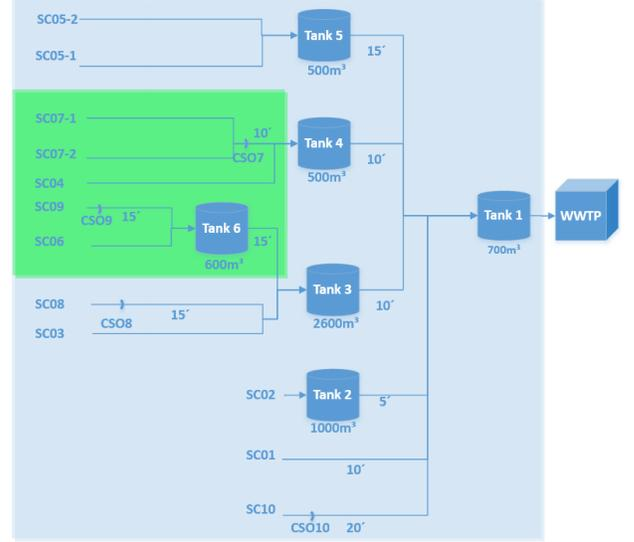
Fig. 2. Astlingen UDS [43] with interconnections between tanks, CSO pipes, WWTP, and pipe delays  $x'$  in minutes. The creek receives CSOs come from the green section and the river receives CSO from the blue section.
