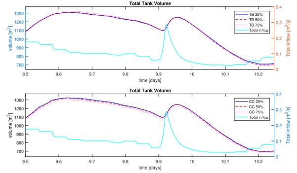
Fig. 3. Volume of T-MPC and CC-MPC with uncertainty bounds 25%–75%.
