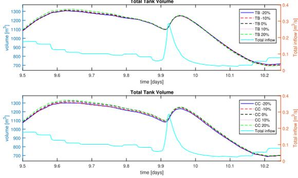
Fig. 4. Volume in tanks of T-MPC and CC-MPC with different scales.
