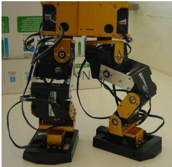
Figure 8: A prototype showing the 6th degree of freedom added to the Robonova platform.
