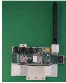
(b) Detail of the interior of the backpack with the embedded PC and the battery hole.
