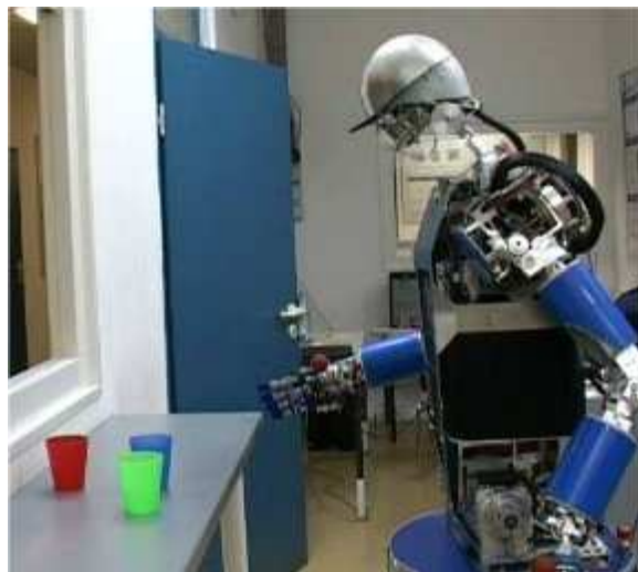
Figure 1: ARMAR-III humanoid robot, from Karlsruhe University, autonomously learning the rules to manipulate objects while avoiding collisions.
