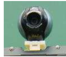
(b) Camera placed on the pan & tilt unit used to perceive the surrounding environment.
