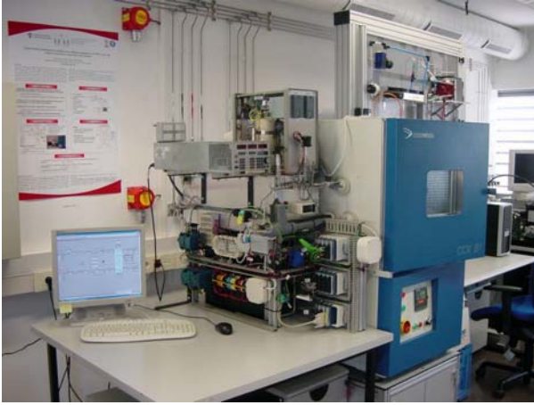
Fig. 1. Picture of fuel cell test station with the environmental chamber.
