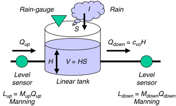
Figure 1 | Virtual reservoir model of a catchment.
