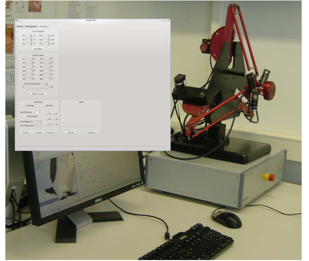
Fig. 2. Delta Haptic Device, whose end-effector is the knob in the middle. The superimposed image shows a snapshot of the GUI.
