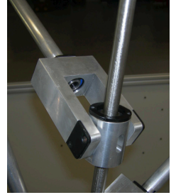
Fig. 10. Prototype of the reconfigurable quadratically-solvable pentapod and its joint implementations.
