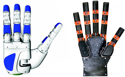
Fig. 1. Different robotic hand designs, the Schunk Anthropomorphic hand, based on the DLR II hand, with four fingers (left), and THE first hand developed at the Centro E. Piaggio with five fingers (right).
