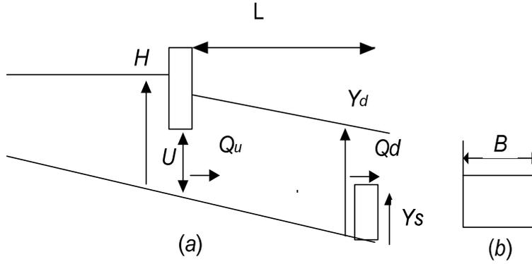
Figure 2. Canal scheme.(a) Longitudinal and (b) cross section.
