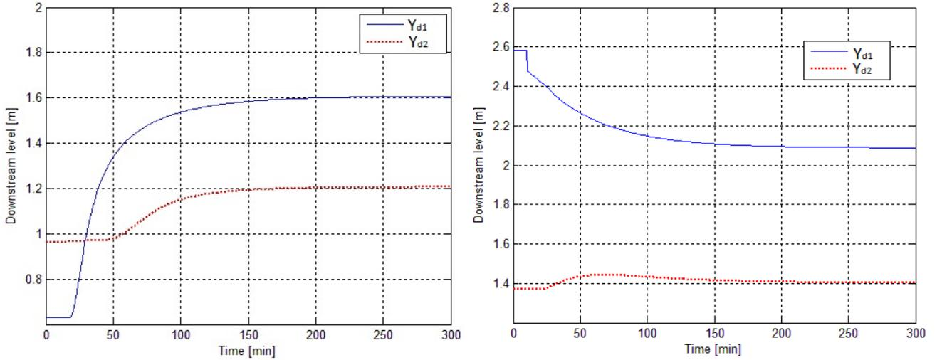
Figure 6. Step time responses for different operating points in two-pool canal. (Left) ( $U_1$  from 0.1 to 0.3m and  $U_2$  remains at 0.5m), (Right) ( $U_1$  remains at 0.5m and  $U_2$  from 0.5 to 0.7m),
