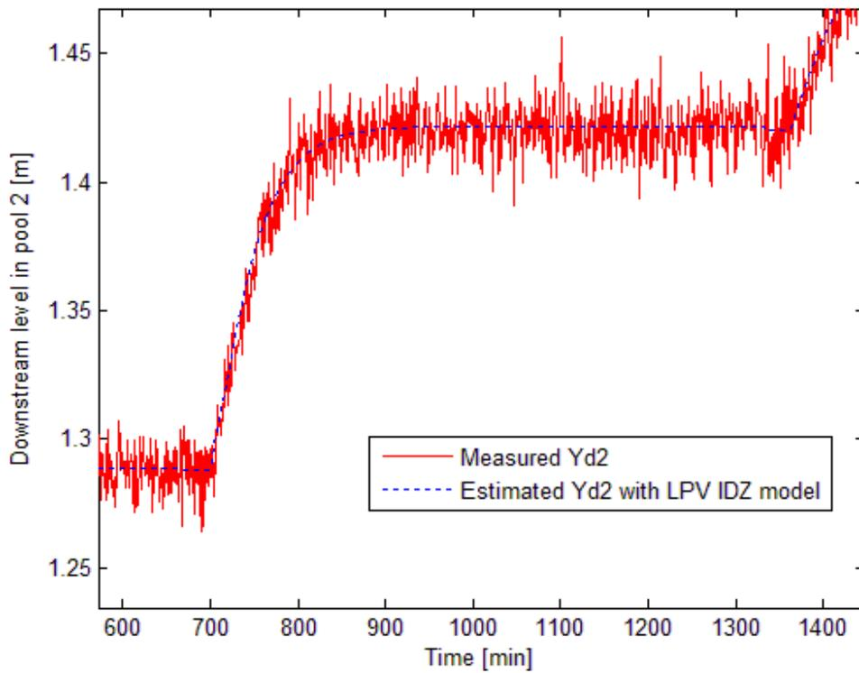
Figure 10. Comparison between the measured and estimated temporal responses in two-pool canal in a scenario that sweeps all the operation range, in right details of the graphics of the left.
