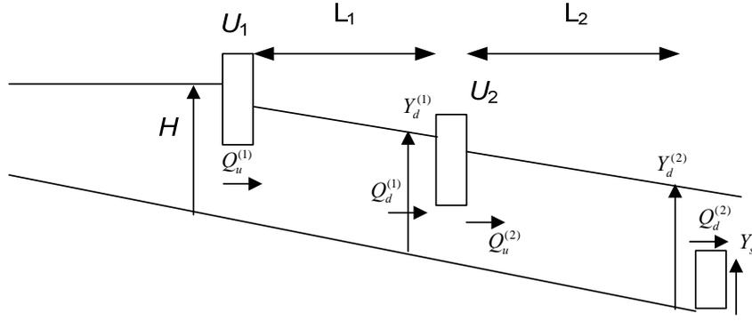
Figure 3. Two-pool canal system
