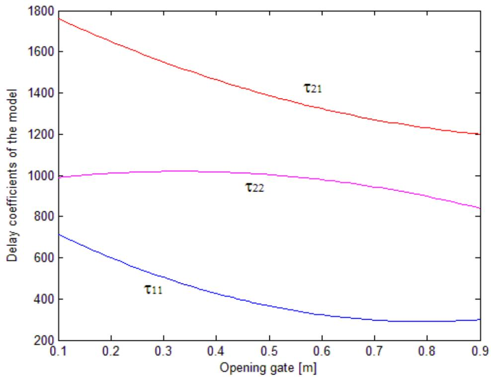
Figure 9. Evolution of the variable parameters of the MIMO model. (Up) gain, (middle), time constant and (down) delay coefficients of the model.
