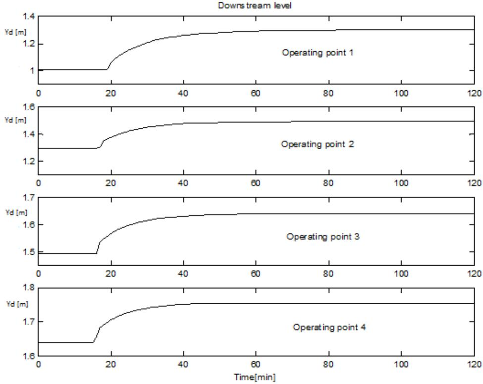
Figure 4. Time response to an opening gate step applied at  $t=10$  min for the four operating points: 1 ( $\theta$  from 0.1 to 0.3m), 2 ( $\theta$  from 0.3 to 0.5m), 3 ( $\theta$  from 0.5 to 0.7m) and 4 ( $\theta$  from 0.7 to 0.9m) that cover of all system operation range.
