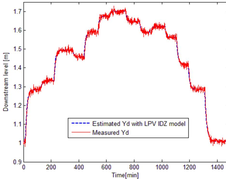
Figure 8. Comparison between the measured and estimated rich temporal responses in SISO case in a scenario model in a scenario that sweeps all the operation range.
