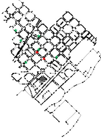
Figure 1 Water network of Nova Icaria DMA (EPANET model) highlighting inner pressure sensors (green stars) and DMA inlets (red triangles)
