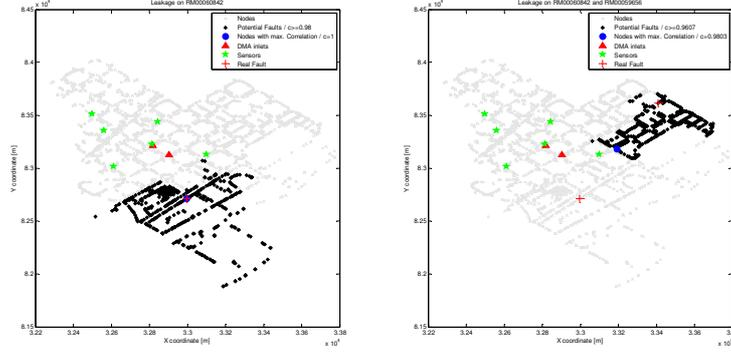
Figure 2 Performance of the direct modeling method using a simulated single-leak scenario (on the left) and a scenario where an extra simulated leak has been added (on the right). The leak exact locations (red cross), the most correlated location predicted by the method (blue spot) and other locations presenting also high correlations (> 98% of the highest correlation) have been highlighted.
