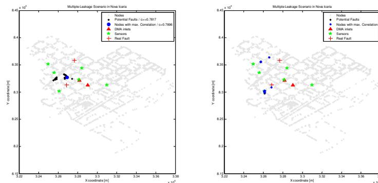
Figure 5 Performance of the direct modeling method (on the left) and the hybrid inverse/direct modeling method (on the right) using real multiple-leak scenario and highlighting the leak exact locations (red cross), the most correlated locations predicted by the methods (blue spot) and other locations presenting also high correlations (> 98% of the highest correlation).
