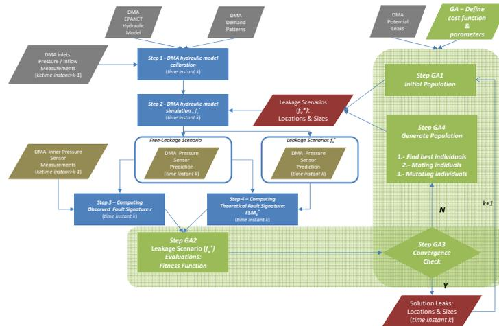
Figure 3 Conceptual scheme of the procedure followed by the leakage location GA-based inverse / direct modeling method at time instant  $k$  highlighting in green those new steps required for the GA-based optimization process.
