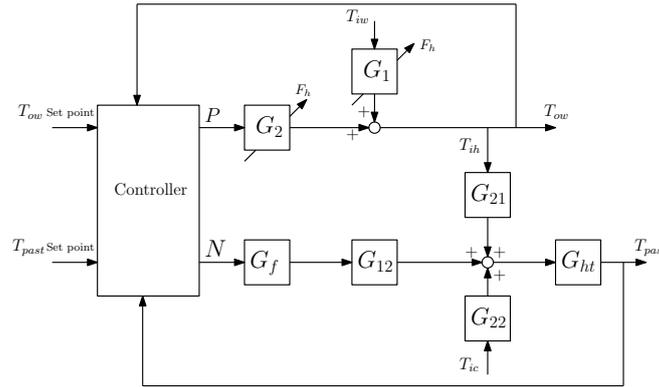
**Figure 6.** Block diagram of the control loop.
