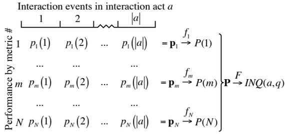
Figure 3: Derivation of interaction quality  $INQ(a, q)$  for an interaction act  $a$  when performing task  $q$ .  $N$  metrics are used to compute performance related to both robot and human. Fusion of performance is done first at event, and then at metric level by the functions  $f_i$  and  $F$  respectively.
