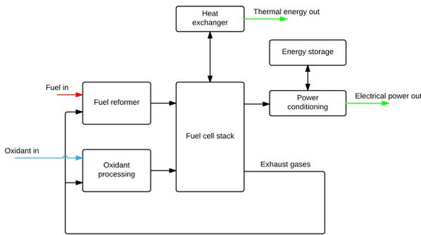
Figure 4: CHP system diagram
