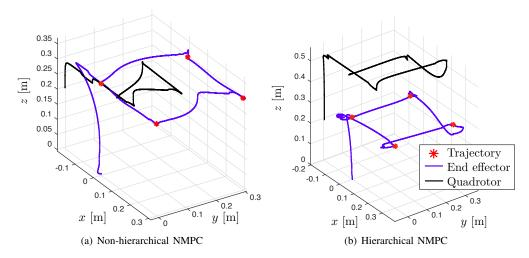
Fig. 6. Simulation results for 3D trajectories, done by the arm end effector using only the positioning task (non-hierarchical) or adding a secondary task (hierarchical) to vertically align the arm CoG and improve the platform flight behavior. In both cases the main task consists in following 4 desired waypoints with the arm end effector.
