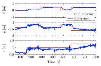
Fig. 7. Real arm end effector positions during a trajectory following task and using the hierarchical NMPC, with the arm CoG alignment as secondary task. The arm end effector position (blue line) has been obtained using a motion capture system.
