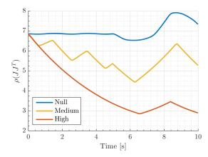
Fig. 4. Behavior of the conditioning number  $\rho_{J_{e,q}}$  in three different experiments, differing in the weight assigned to the conditioning number cost function. The red line represents the experiment with larger assigned weight, achieving a smaller  $\rho_{J_{e,q}}$ , whereas the blue line is the result of the experiment with zero weight assigned to the cost function, thus not reducing  $\rho_{J_{e,q}}$ .
