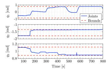
Fig. 8. Arm joint positions  $(q_i)$  during the same trajectory following task and hierarchical NMPC as in Fig. 7. The horizontal dashed lines correspond to lower and upper bounds of a constraint, set to avoid self-collisions.
