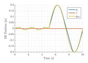
Fig. 2. End effector trajectory compared with the reference signal. Notice how the z reference is not reported because it is always null.
