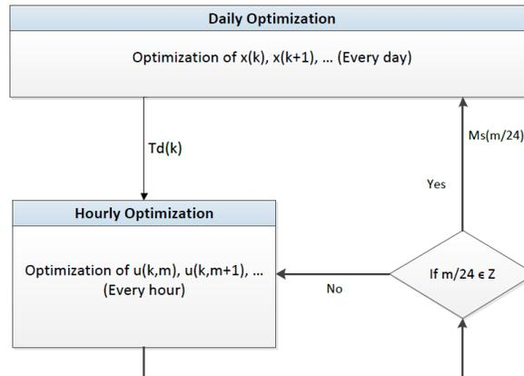
**Fig. 1** Optimizations of multi-layer MPC
