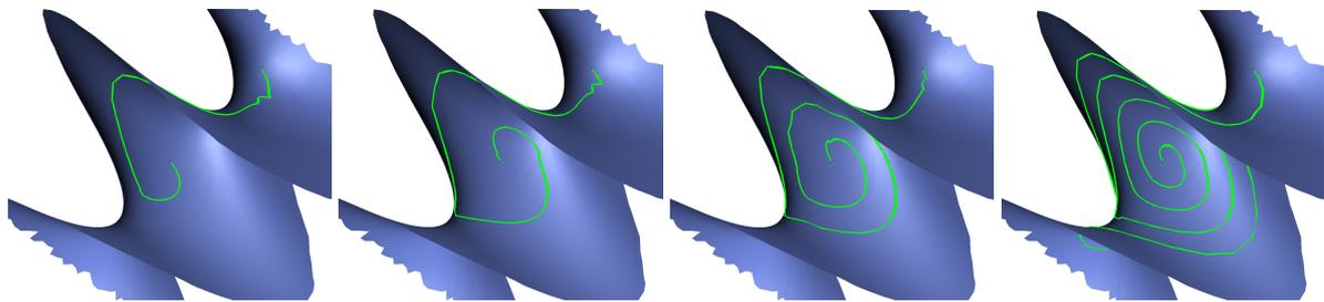
**Figure 6:** From left to right, the state manifold (in blue), and the trajectory obtained (green) for a maximum torque  $\tau_{max}$  of 16, 12, 8, and 4 [Nm].
