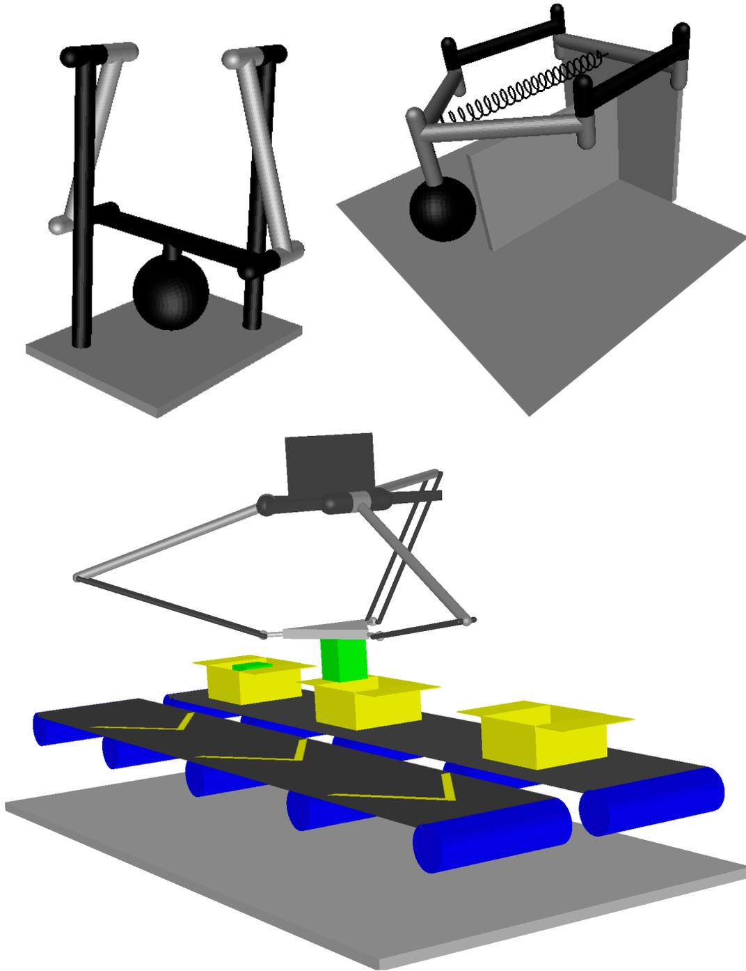
**Figure 5:** Test cases used to validate the planner: a four-bar pendulum (-left), a five-bar robot (top-right), and a Delta robot (bottom).
