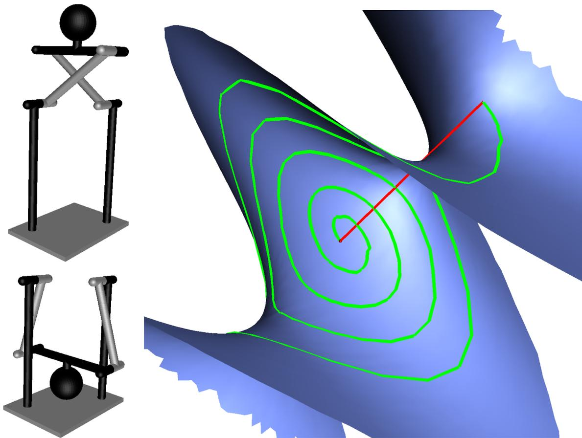
**Figure 1:** A kindodynamic planning problem on a four-bar pendulum modeling a swing boat ride. Left: The start and goal states, both with null velocity. Right: The kinematic constraints define an helicoidal manifold. A kinematically-feasible trajectory (red) and a trajectory also fulfilling dynamic constraints (green) may be quite different.
