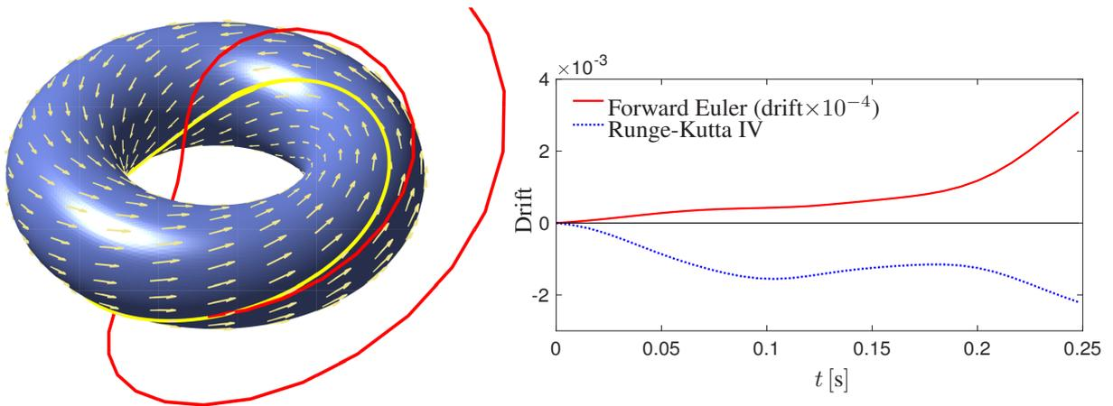
**Figure 2:** Drift caused by numerical integration of an ODE system. Left: A particle moving on a torus under the shown vector field. The trajectory obtained by the forward Euler method (red) increasingly diverges from the exact trajectory (yellow). Right: With more accurate procedures, such as the 4th order Runge-Kutta method (blue), the drift may be reduced, but not canceled.
