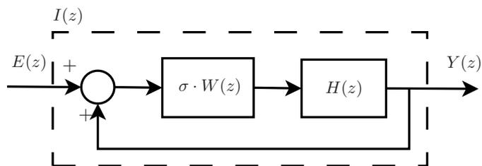
Figure 1. Internal model used in Repetitive Control.
