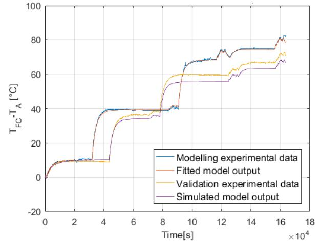
Fig. 3: Experimental and model curves (open windows)
