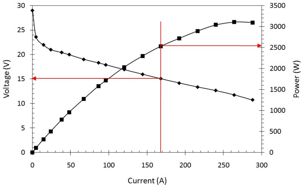
Figure 2. Polarization curve obtained for the 30-cells stack operating under optimal conditions
