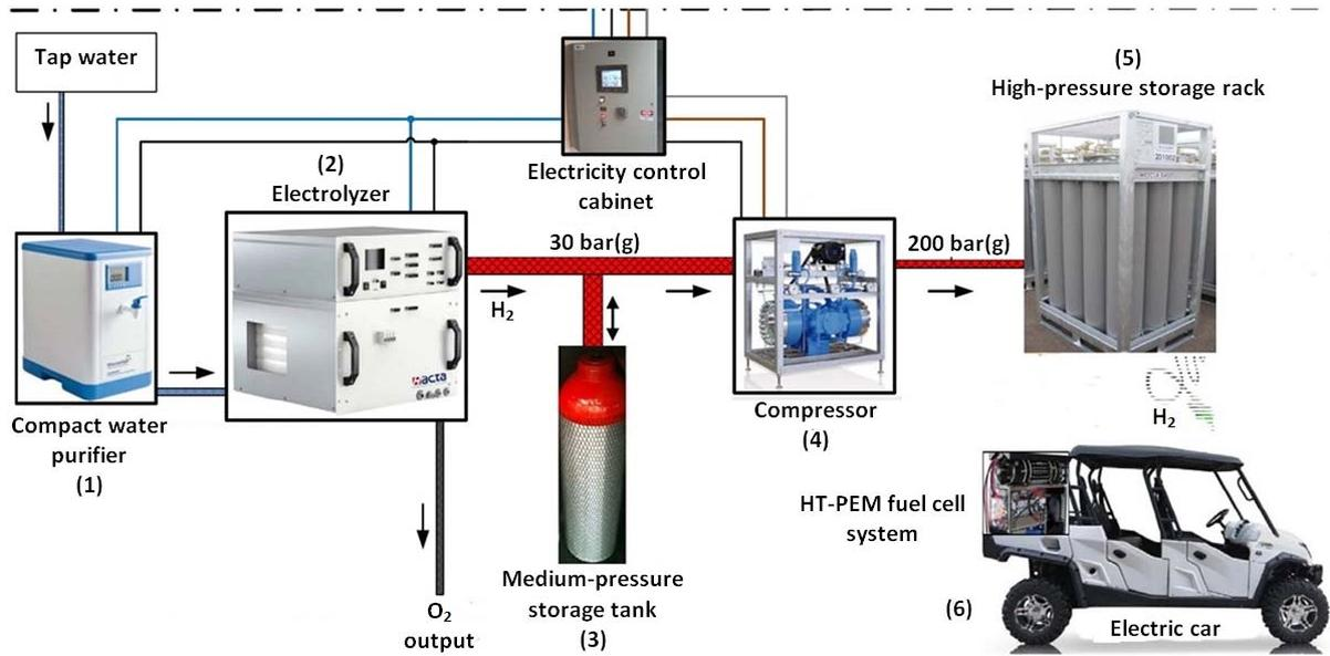
Figure 1. General scheme of the hydrogen production and storage plant together with the end-user commercial electric vehicle properly modified to be powered by a hybrid powertrain
