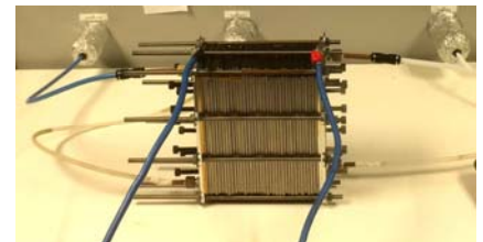
Figure 4. 35-cells high-temp PEMFC manufactured at LIFTEC
