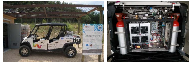
Fig. 1. Photos of the modified electric car with the fuel cell system assembled at the tilting rear load platform
