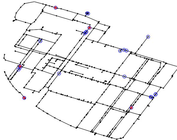
Fig. 6: DMA network sensor placement results under sensitivity analysis approach
