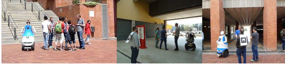
Figure 1: Dabo performs the search-and-track task with a target (wearing a tag for recognition) in different urban environments.
