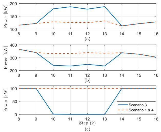
Fig. 2. The operation of sub-system 3 and 2 in Scenario 3 (solid lines) and Scenario 1 & 4 (dashed lines). (a) Power generated by sub-system 3 ( $p_3^{\text{g}}$ ), (b) Power generated by sub-system 2 ( $p_2^{\text{g}}$ ), and (c) Power transferred from sub-system 2 to sub-system 3 ( $p_{32}^{\text{t}}$ ).
