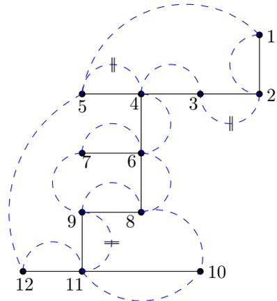
Fig. 1. The microgrids (dots) in their electrical network  $\mathcal{G}$  (solid lines) and information-sharing network  $\hat{\mathcal{G}}$  (dashed lines). The double lines,  $\parallel$ , indicate the broken links during communication failures in the simulations.
