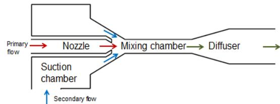
Figure 2. Ejector schematic.
