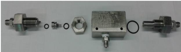
Figure 1. Parts of the experimental ejector.
