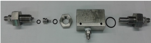
Figure 1. Parts of the experimental ejector.
