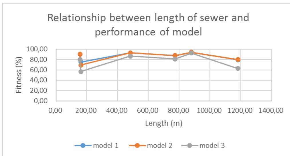
Figure 4 Relationship between sewer length and model performance
