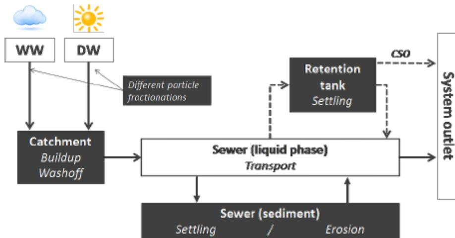
Figure 1 New Structure of Quality Module SWMM-TSS
