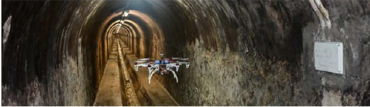
Fig. 3. Quadrotor flight in Passeig Sant Joan in Barcelona, a real sewer environment.
