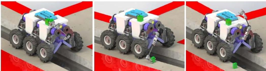
Fig. 2. SIAR Robot deploying one wifi communication repeater.
