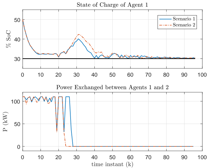
FIGURE 5 The evolution of SoC of agent 1 (top plot) and the power exchanged between agent 1 and its adversarial neighbor, agent 2 (bottom plot).
