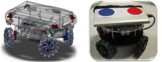
Fig. 1. Four-wheeled omni-directional mobile robot [19].
