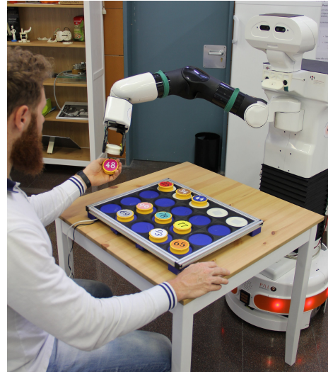
Fig. 1: Tiago robot interacting with a user while he is playing a cognitive exercise. The initial policy of the robot has been generated learning the user's profile using the Persona-Behaviour Simulator.
