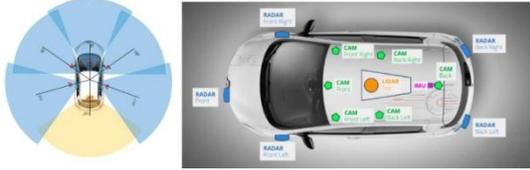
Figure 3: Sensor disposition of the used Nuscenes dataset [3]
