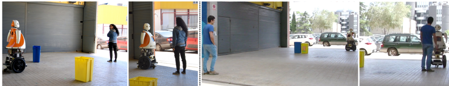
Fig. 1: The robot uses the implemented method to approach a static and moving person, while avoiding several static obstacles of the environment.
