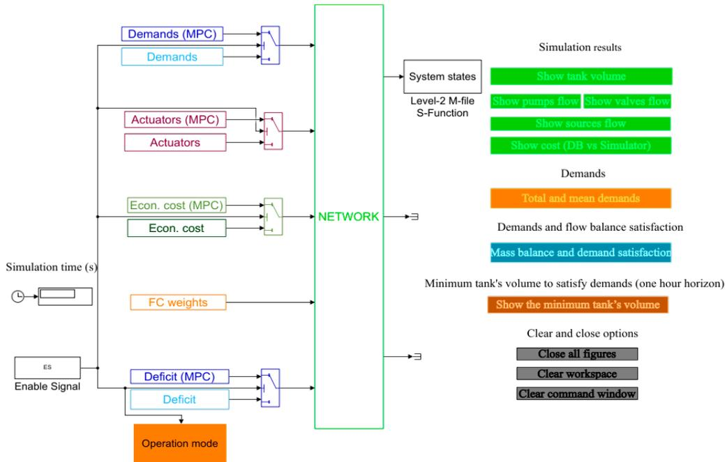
Figure 5. Digital representation of Barcelona WSS using MATLAB/SIMULINK.
