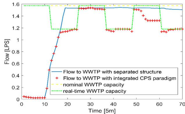
**Figure 12.** Comparisons of the flow from WSCS to WWTP in Scenario 1 (blue) and Scenario 2 (red).
