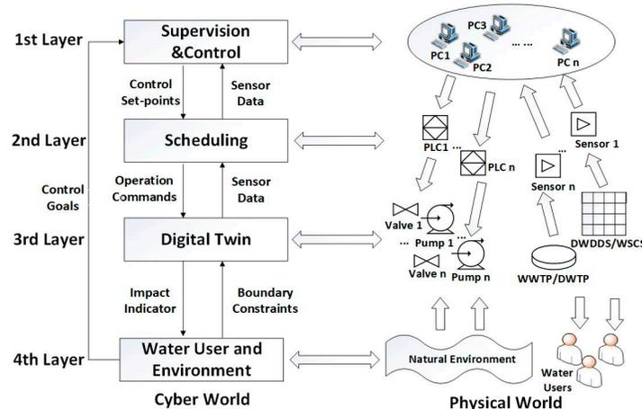
**Figure 2.** Multilayer cyber-physical system (CPS)-based supervision structure.
