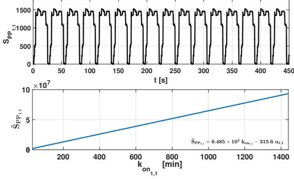
Fig. 3. Energy consumption profile and correlation for  $PP_{1,1}$ .
