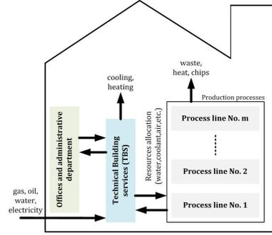
Fig. 1. Representation of a manufacturing plant and its constitutive elements. Based on Duflou et al. (2012).
