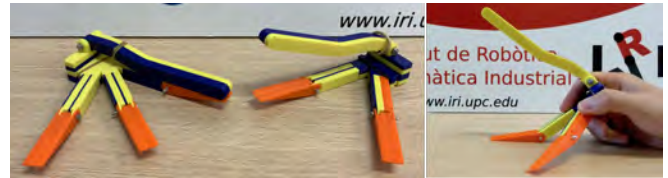
Fig. 3. Simple prototypes to evaluate the grasp geometries.
