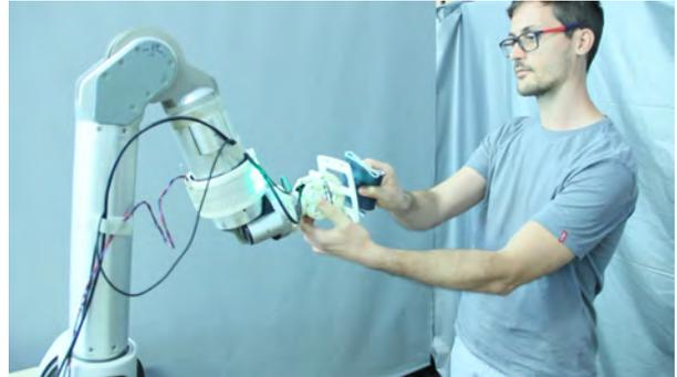
Fig. 1: Industrial scenario considered in this task. The operator can polish, grab the object or move the robot actuating over the shared object. Samples from the force sensor are used to classify user intentions, which change the robot behavior adaptively.
