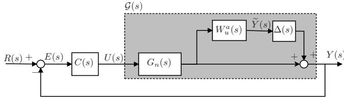
Fig. 4. Closed-loop scheme with a plant with multiplicative uncertainty.
