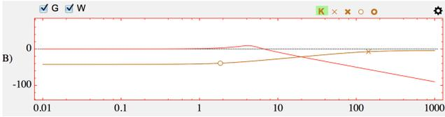
Fig. 10. Example:  $G_n(s)$  and  $(W_u^a)^{-1}$  magnitude Bode diagrams as seen in RCLSD ( $G_n(s)$  in red,  $(W_u^a)^{-1}$  in brown).
