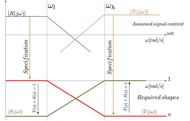
Fig. 2. Signal frequency decomposition and desired frequency responses.
