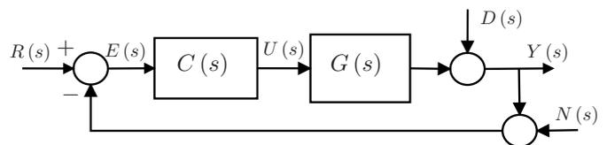
Figure 1. Closed-loop control system block diagram.
