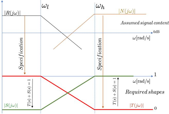
Figure 2. Signal frequency decomposition and desired frequency responses.
