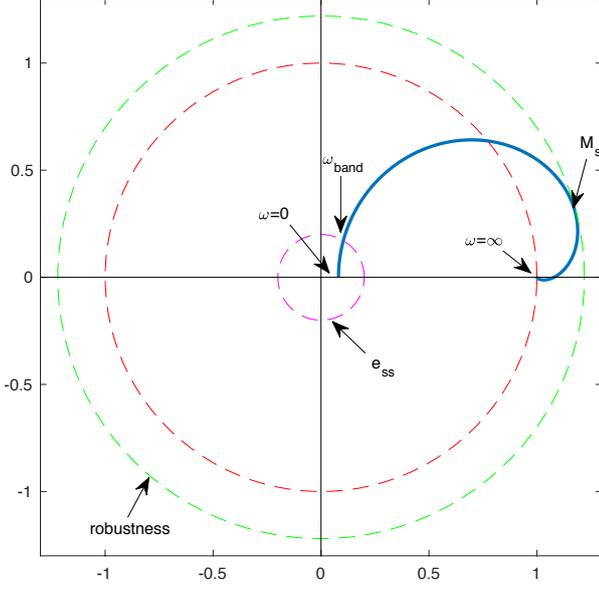
Figure 5. Sensitivity function specifications over the polar diagram.
