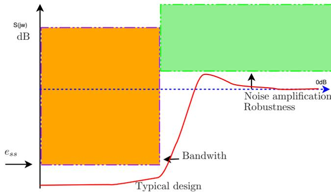
Figure 4. Bode plot Sensitivity function specifications.
