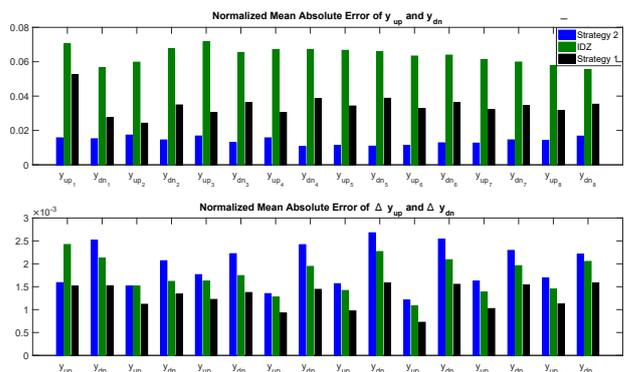
Fig. 8. Normalized mean absolute errors between the reference model and the modeling approaches for the eight pools.
