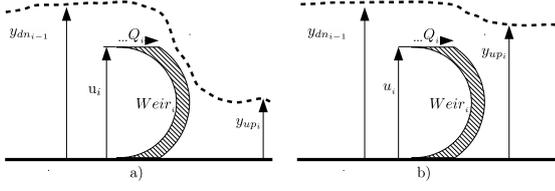
Fig. 3. Flow relation for: a) Weir in free-flow. b) Weir in submerged-flow.
