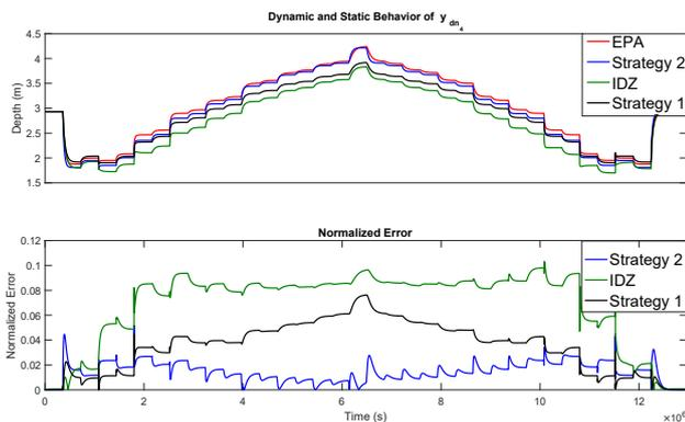
Fig. 6. Comparison of the behavior of the simulated systems at the downstream level of the fourth channel.
