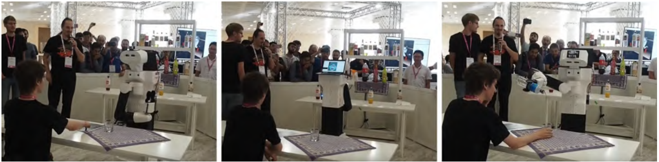
Fig. 4: Snapshots of demo execution for the TAMS team. From left to right: user pointing to the menu for choosing a drink, TIAGo moving to the bar for retrieving one of the required liquors, and TIAGo pouring the (real) liquor on the glass.
