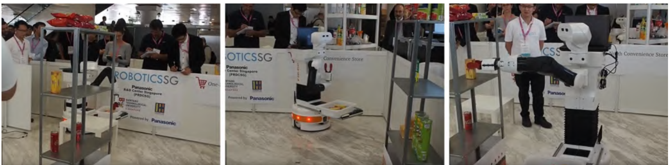
Fig. 5: Snapshots of demo execution for the Robotics.SG team. From left to right: TIAGo retrieving the bin with the returned items, TIAGo navigating the store using a pre-recorded map, and TIAGo placing one of the items on the required shelf.
